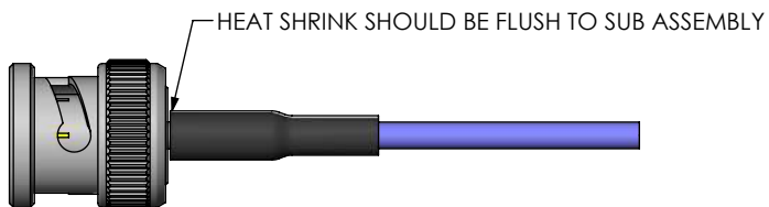
IN-PROCESS 5 ACTIVATE HEAT SHRINK
