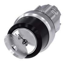
RONIS key-operated switch, 22 mm, round, metal, shiny, lock number SB30, with 2 keys, 2 switch positions O-I, latching, actuating angle 90°, 10:30h/13:30h, key removal O+I, possible special locks: SB31, 421, 455, with laser labeling, upper case and lower case, always upper case at beginning of line
