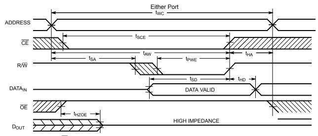
Write Cycle No. 2 (R/W Three-States Data I/Os—Either Port)<sup>[16, 23]</sup>
