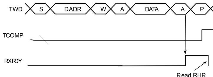
**Figure 28-11.** Slave Receiver with Multiple Data Bytes
