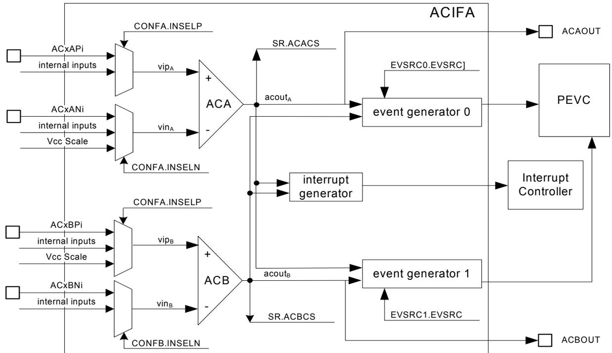
Figure 35-2. Analog Comparator Interface in window mode
