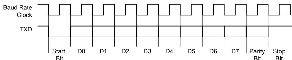
The characters are sent by writing in the Transmit Holding Register (THR). The transmitter reports two status bits in the Channel Status Register (CSR): TXRDY (Transmitter Ready), which indicates that THR is empty and TXEMPTY, which indicates that all the characters written in THR have been processed. When the current character processing is completed, the last character written in THR is transferred into the Shift Register of the transmitter and THR becomes empty, thus TXRDY rises.
