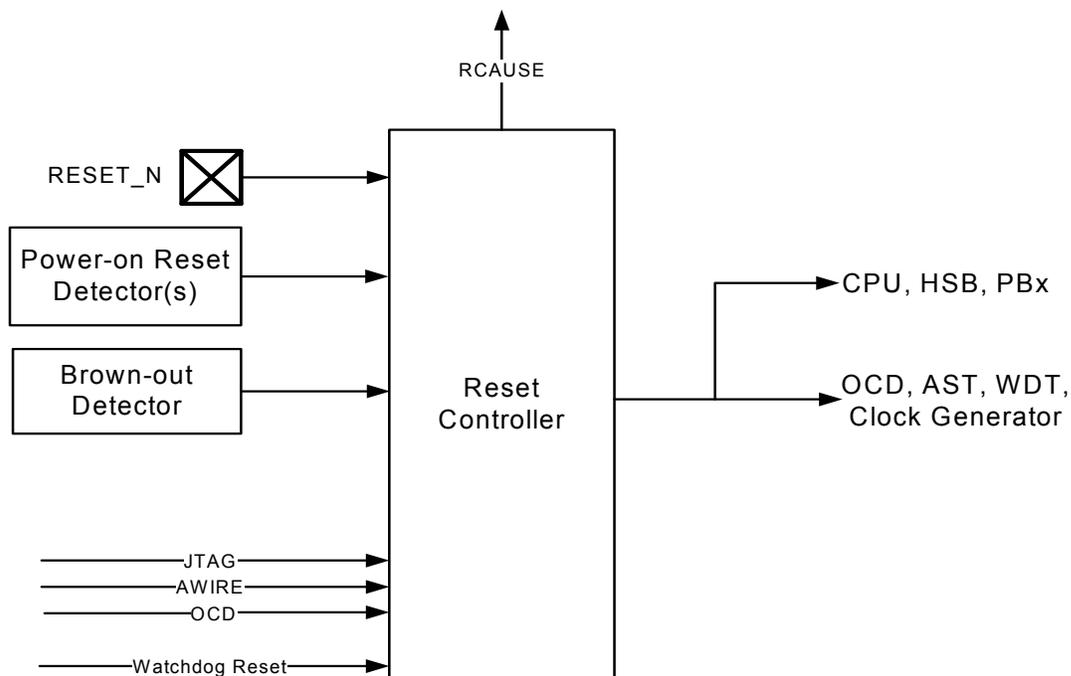
In addition to the listed reset types, the JTAG & aWire can keep parts of the device statically reset. See JTAG and aWire documentation for details.
