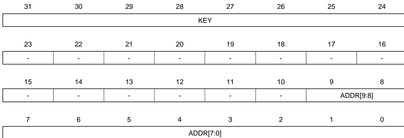
To unlock a write protected register, first write to the UNLOCK register with the address of the register to unlock in the ADDR field and 0xAA in the KEY field. Then, in the next PB access write to the register specified in the ADDR field.
