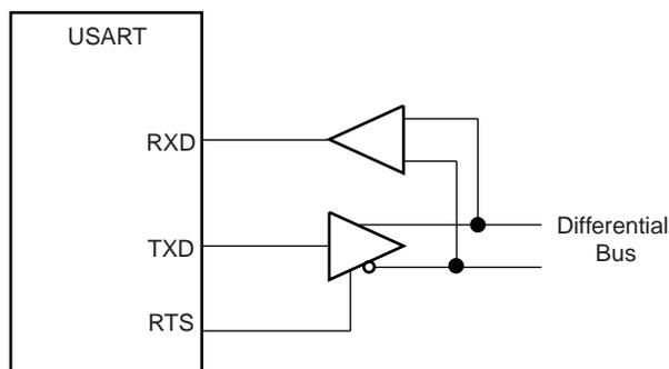
The USART is set in RS485 mode by programming the MODE field in the Mode Register (MR) to the value 0x1.
