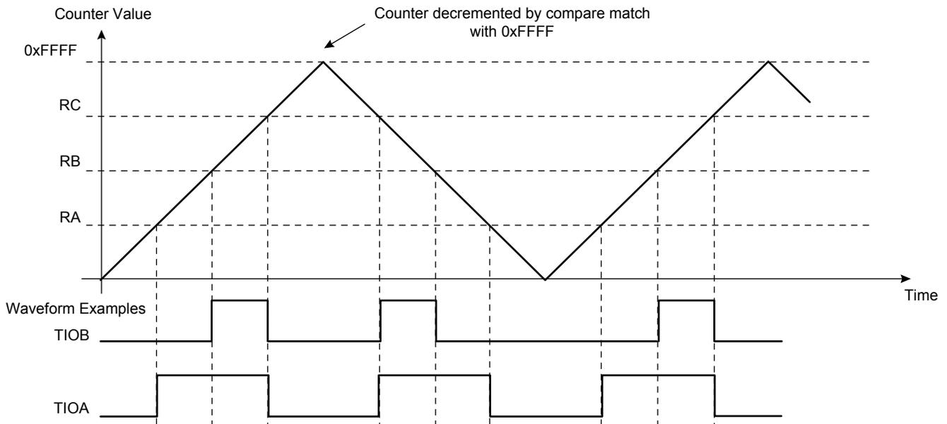
**Figure 31-11. WAVSEL = 1 With Trigger**
