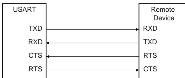
Setting the USART to operate with hardware handshaking is performed by writing the MODE field in the Mode Register (MR) to the value 0x2.
