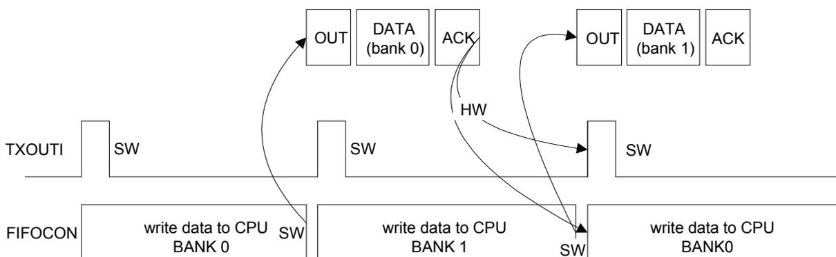
**Figure 32-23.** Example of an OUT pipe with two data banks and a bank switching delay
