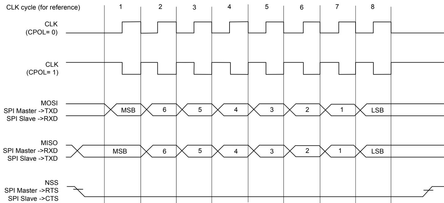
Figure 25-38. SPI Transfer Format (CPHA=0, 8 bits per transfer)
