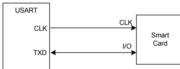
When operating in ISO7816, either in T = 0 or T = 1 modes, the character format is fixed. The configuration is 8 data bits, even parity and 1 or 2 stop bits, regardless of the values programmed in the CHRL, MODE9, PAR and CHMODE fields. MSBF can be used to transmit LSB or MSB first. Parity Bit (PAR) can be used to transmit in normal or inverse mode. Refer to ["Mode Register" on page 627](#) and ["PAR: Parity Type" on page 629](#).
