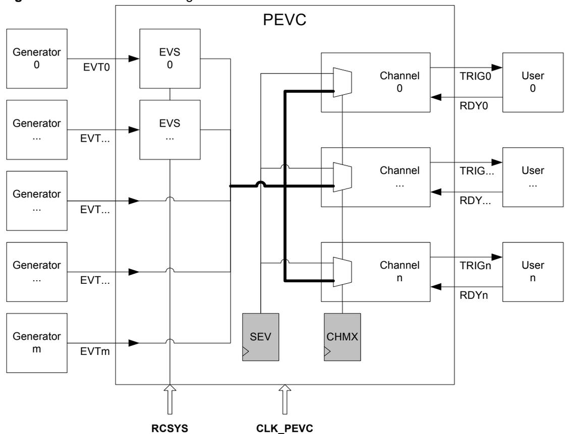
The maximum number of generators, Event Shapers, channels, and users supported by the Peripheral Event Controller is 64. Please refer to the Module Configuration section at the end of this chapter for the device-specific configuration.
