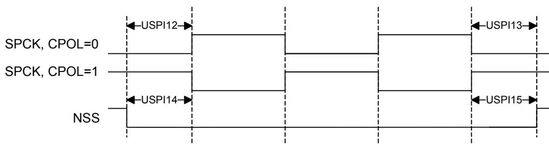
**Table 40-47.** USART in SPI mode Timing, Slave Mode<sup>(1)</sup>
