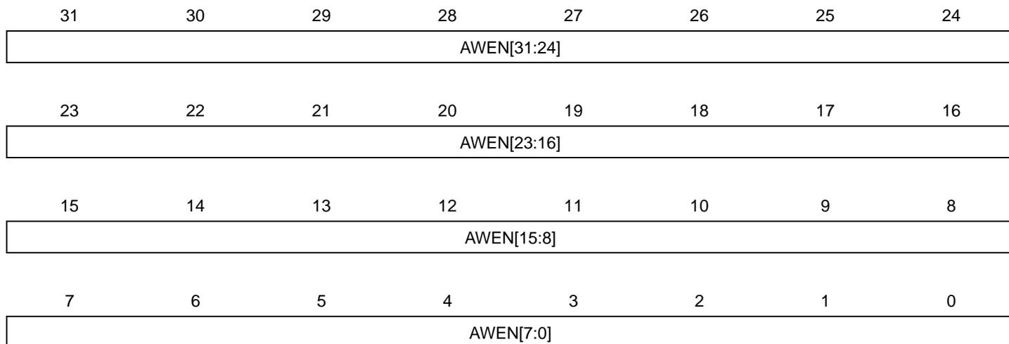
Each bit in this register corresponds to an asynchronous wake up, according to [Table 7-11](#).
