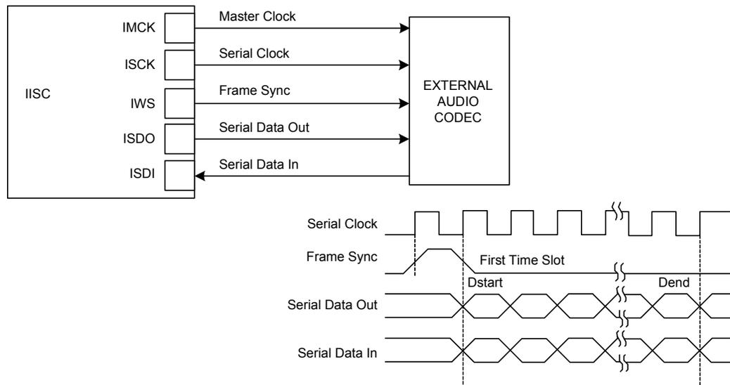
Figure 30-8. Time Slot Application Block Diagram
