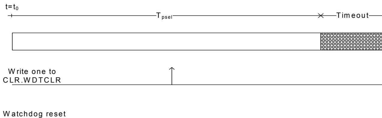
If the WDT counter is not cleared within  $T_{psel}$  a watchdog reset will be issued at the end of  $T_{psel}$ , see [Figure 10-3 on page 164](#).
