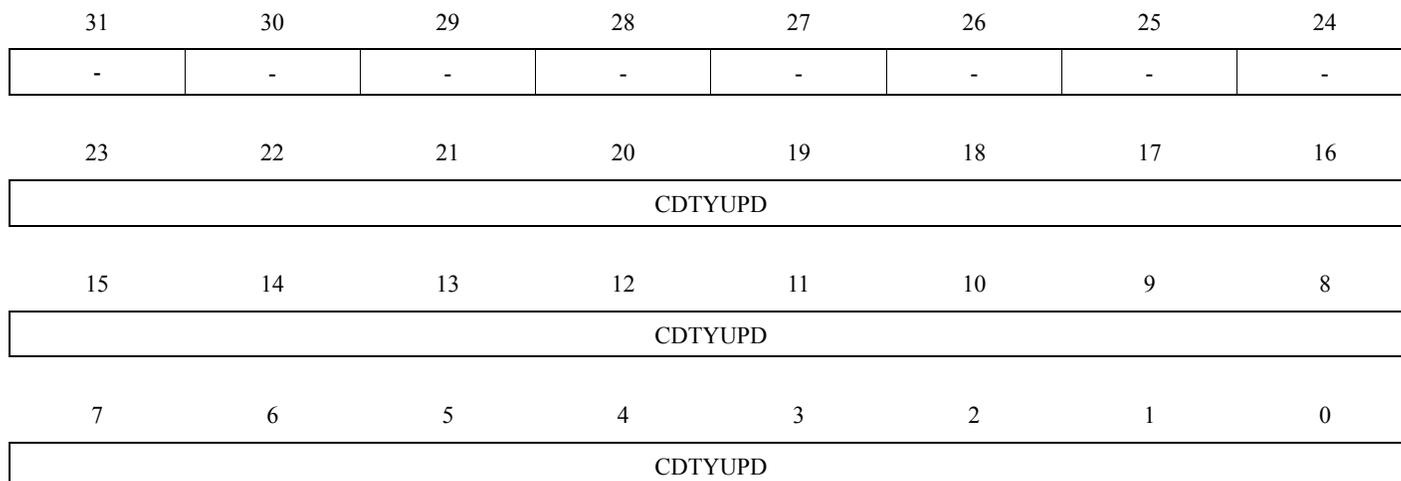
This register acts as a double buffer for the CDTY value. This prevents an unexpected waveform when modifying the waveform duty-cycle.
