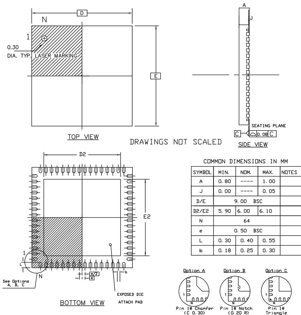
Note: The exposed pad is not connected to anything internally, but should be soldered to ground to increase board level reliability.
