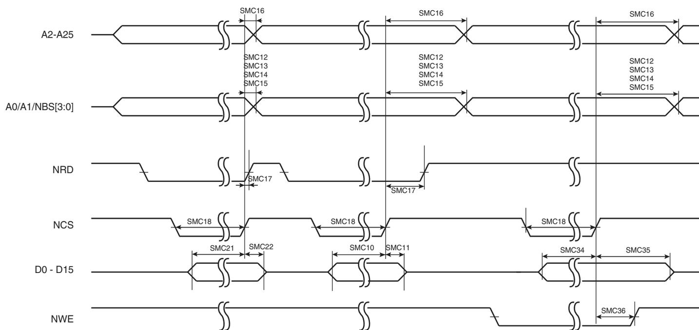
**Figure 40-18. SMC Signals for NRD and NRW Controlled Accesses<sup>(1)</sup>**
