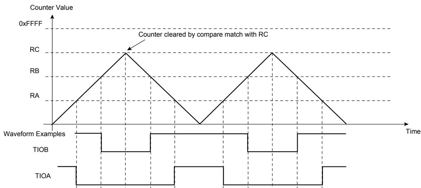
Figure 31-13. WAVSEL = 3 With Trigger
