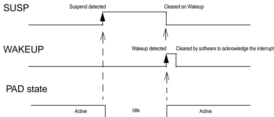
The Suspend Interrupt bit in the Device Global Interrupt register (UDINT.SUSP) is set and the Wakeup Interrupt (UDINT.WAKEUP) bit is cleared when a USB Suspend state has been detected on the USB bus. This event automatically puts the USB pad in the Idle state. The detection of a non-idle event sets WAKEUP, clears SUSP, and wakes the USB pad.
