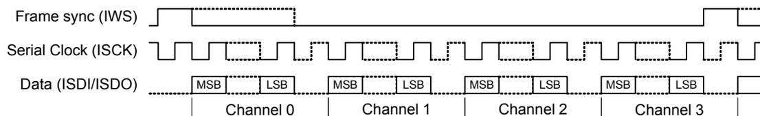
Data bits are sent on the falling edge of the Serial Clock and sampled on the rising edge of the Serial Clock. The IWS pin provides a frame synchronization signal, starting one ISCK period before the MSB of channel 0.
