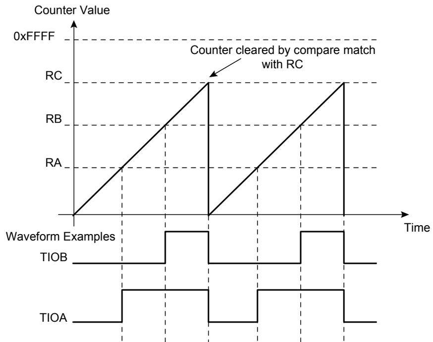
**Figure 31-9.** WAVSEL = 2 With Trigger
