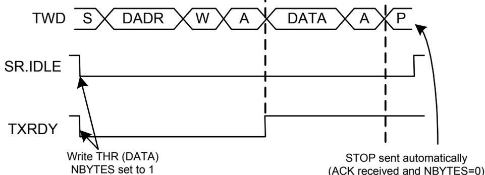
**Figure 27-7.** Master Write with Multiple Data Bytes
