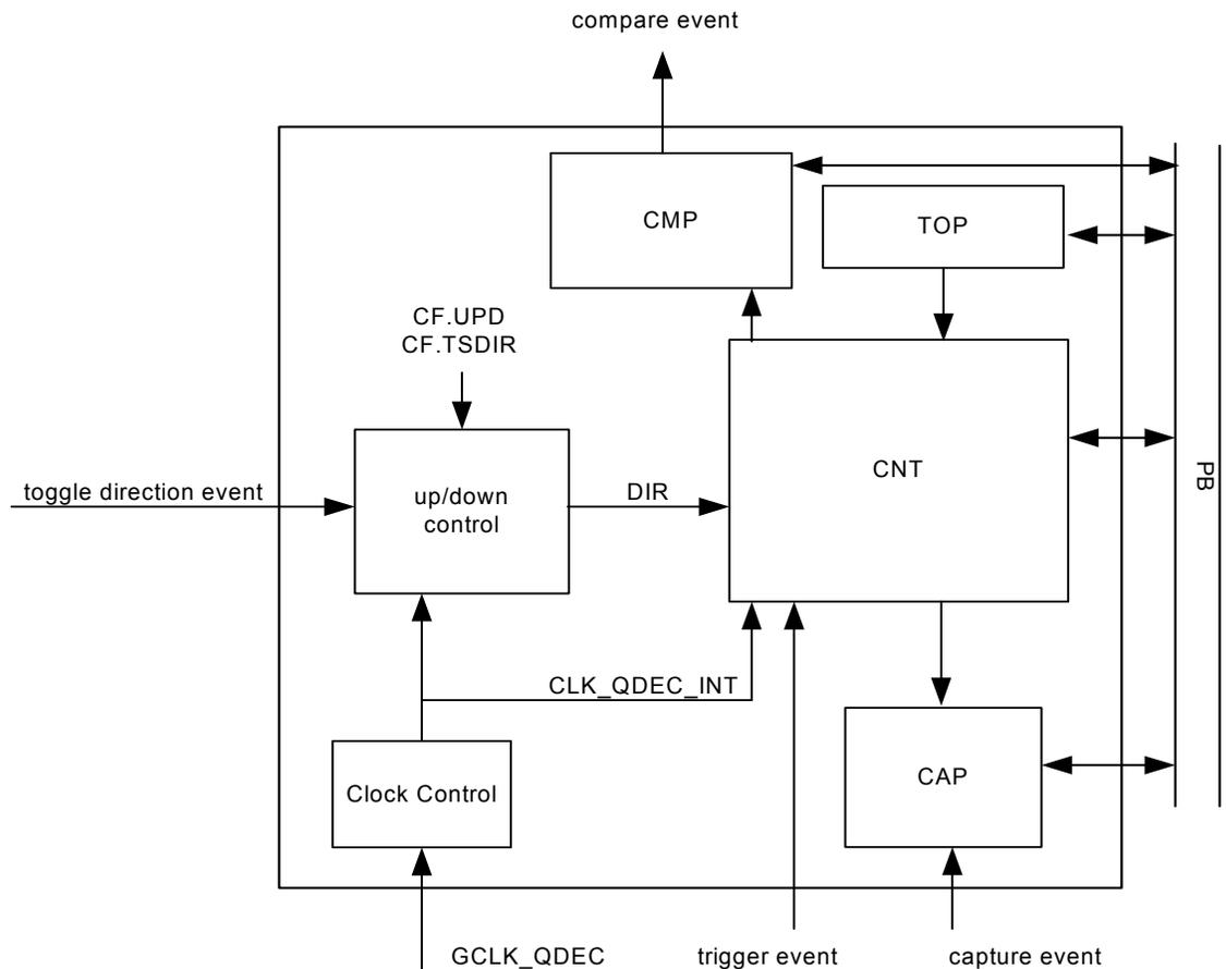
The user can set the timer count direction by writing to the CF.TSDIR bit. The counting direction is taken into account when a trigger occurs. The counting direction is shown in SR.CNTDIR.
