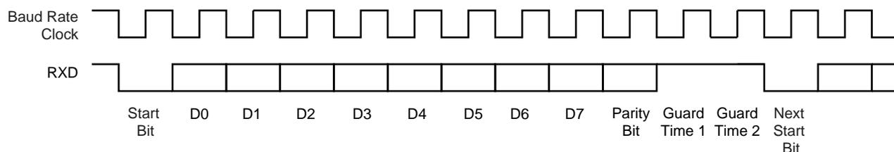
**Figure 25-31.** T = 0 Protocol with Parity Error
