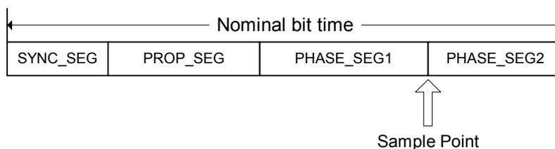
The duration of each time segment is divided into time quanta (TQ). The total number of TQ in a bit time must be in the range [8..25].
