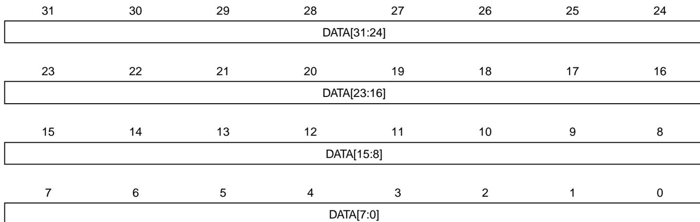
These registers are general purpose 32-bit registers that are reset only by power-on-reset. Any other reset will keep the bits of these registers untouched.
