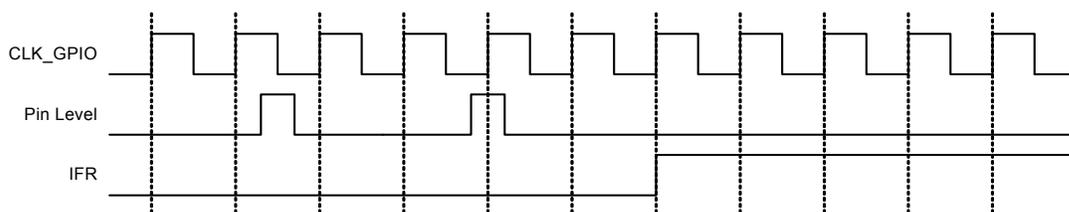
Figure 23-5 shows the timing for rising edge (or pin-change) interrupts when the glitch filter is enabled. For the pulse to be registered, it must be sampled on two subsequent rising edges. In the example, the first pulse is rejected while the second pulse is accepted and causes an interrupt request.
