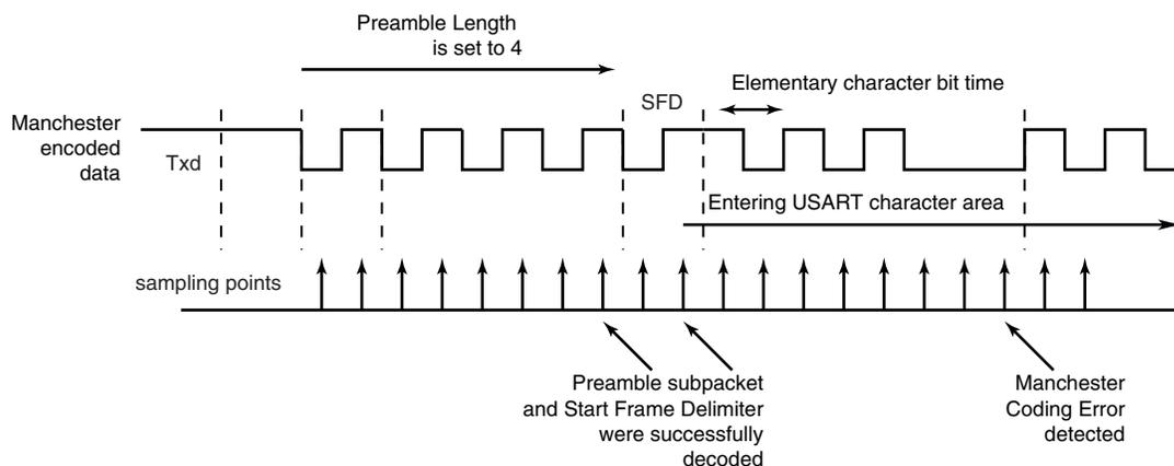
When the start frame delimiter is a sync pattern (ONEBIT field at 0), both command and data delimiter are supported. If a valid sync is detected, the received character is written as RXCHR field in the RHR register and the RXSYNH is updated. RXCHR is set to 1 when the received character is a command, and it is set to 0 if the received character is a data. This mechanism alleviates and simplifies the direct memory access as the character contains its own sync field in the same register.
