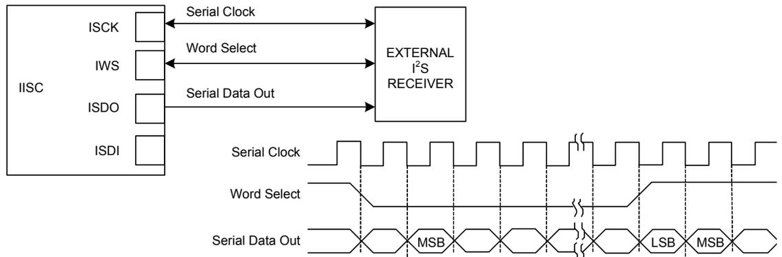
Figure 30-7. Codec Application Block Diagram
