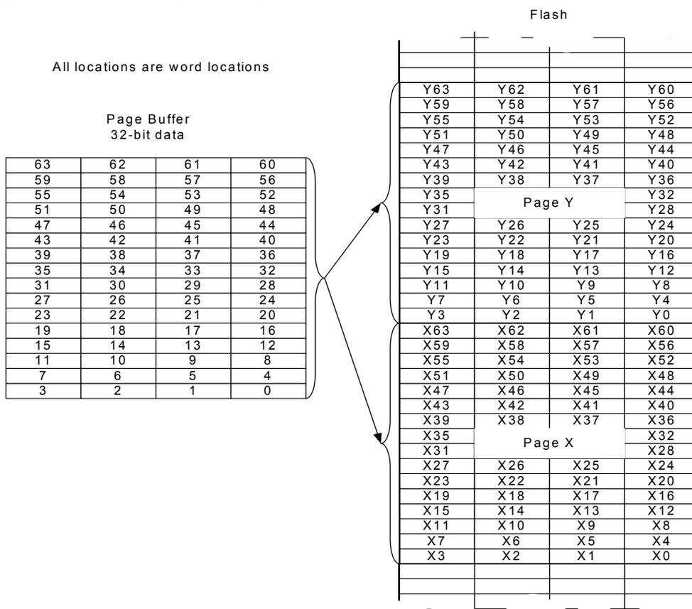
The page buffer is word-addressable and should only be written with aligned word transfers, never with byte or halfword transfers. The page buffer can not be read.
