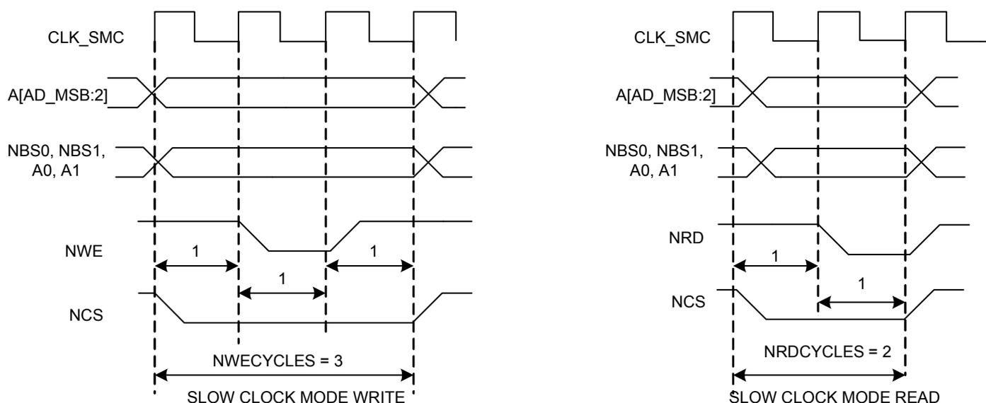
**Table 18-5.** Read and Write Timing Parameters in Slow Clock Mode
