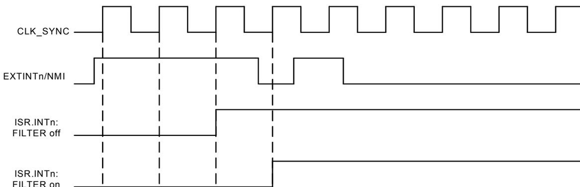
**Figure 12-3.** Timing Diagram, Synchronous Interrupts, Low Level or Falling Edge
