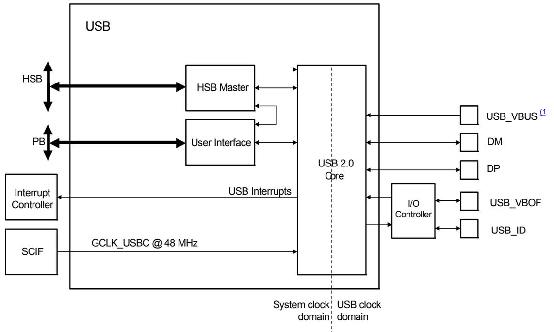
Note: The USB\_VBUS pin is 5V tolerant
