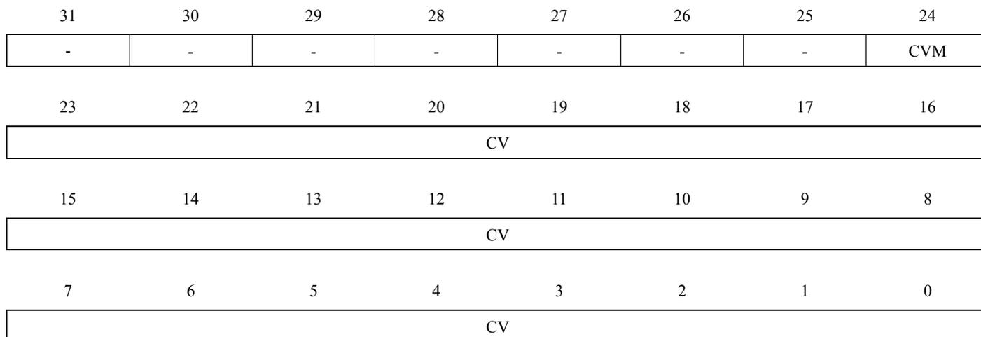
Only the first 20 bits (channel counter size) of CV field are significant.
