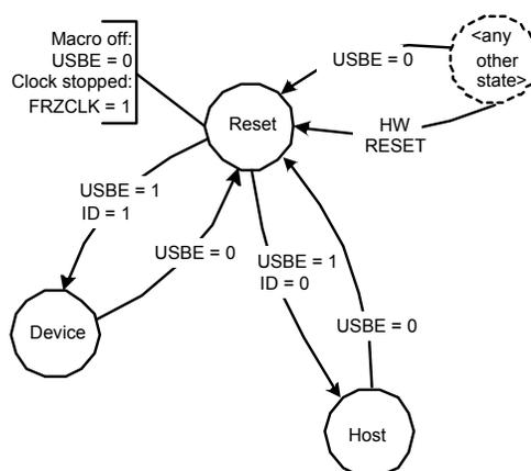
After a hardware reset, the USBC is in the Reset state. In this state:
