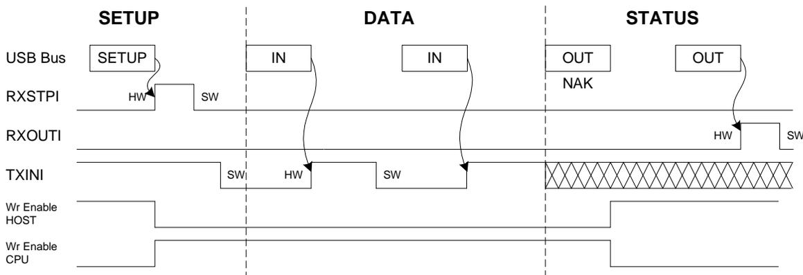
A NAK handshake is always generated as the first status stage command. The UESTAn.NAKINI bit is set. It allows the user to know that the host aborts the IN data stage. As a consequence, the user should stop processing the IN data stage and should prepare to receive the OUT status stage by checking the UESTAn.RXOUTI bit.
