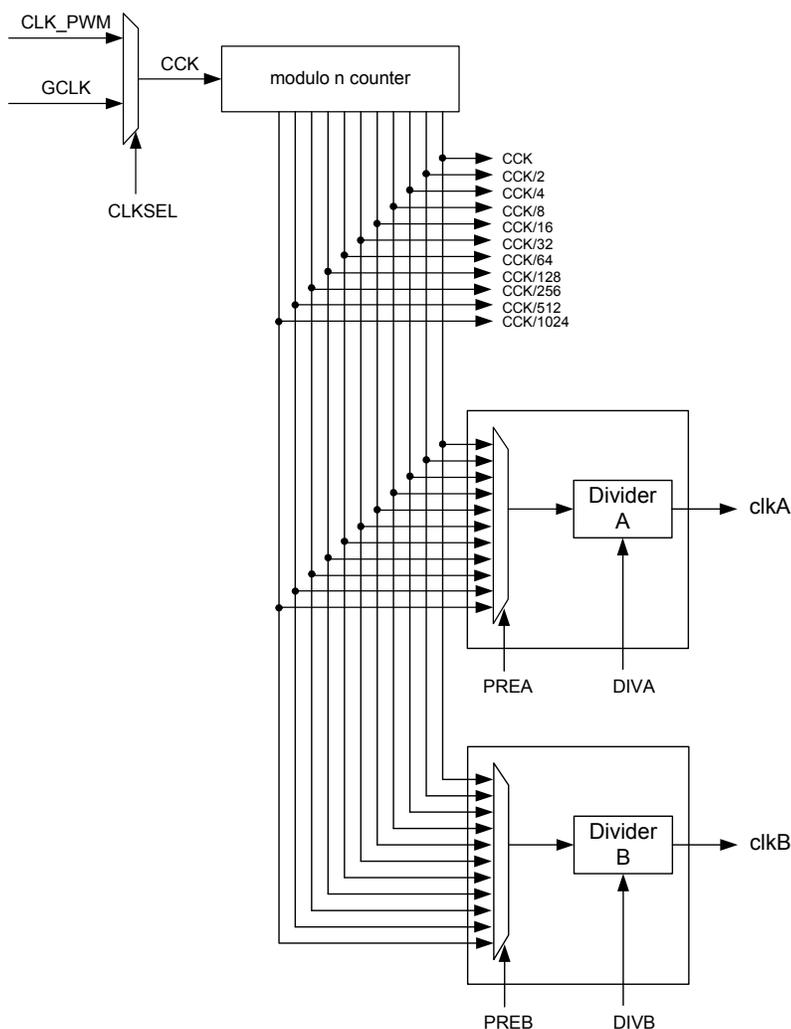
The PWM internal clock (named CCK and driven either by CLK\_PWM or by GCLK) is divided in the clock generator module to provide different clocks available for all channels. Each channel can independently select one of the divided clocks.
