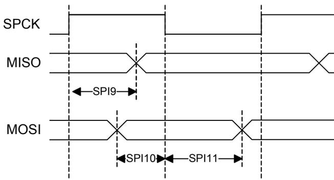
**Figure 40-15.** SPI Slave Mode NPCS Timing
