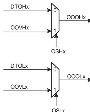
The OSHx and OSLx fields in the "Output Selection Register" on page 1015 (OS) allow the outputs of the dead-time generator DTOHx and DTOLx to be overridden by the value defined in the OOVHx and OOVLx fields in the "Output Override Value Register" on page 1014 (OOV).
