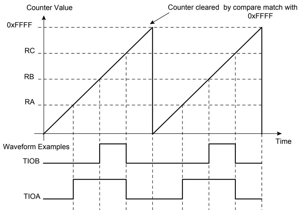
Figure 31-7. WAVSEL= 0 With Trigger
