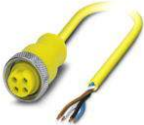
Sensor/Actuator cable, 4-position, PVC, Yellow RAL 1021, Free cable end, on Socket straight 7/8"-16UNF, A-coded, Cable length: 2 m
