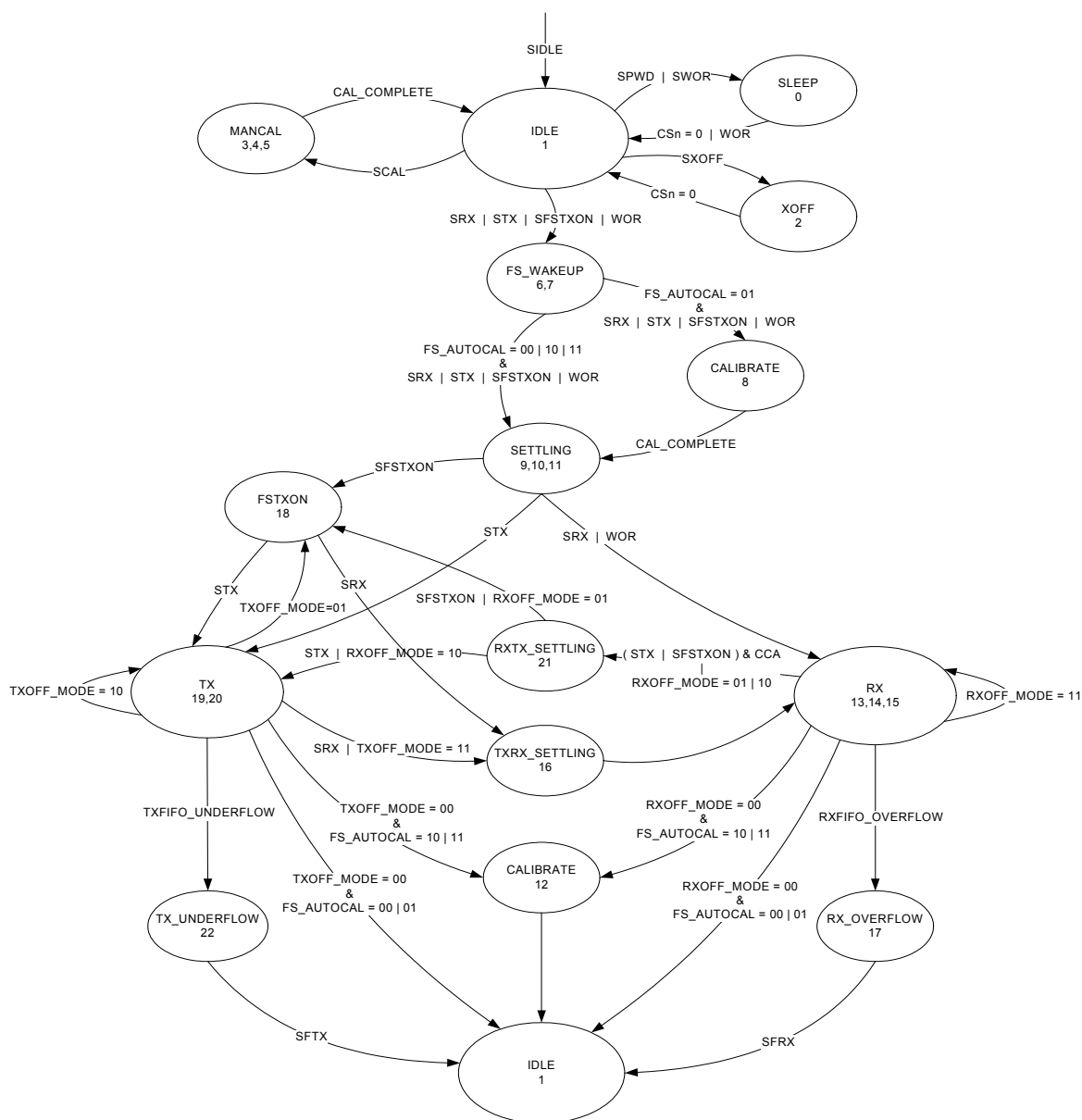
Figure 16: Complete Radio Control State Diagram
