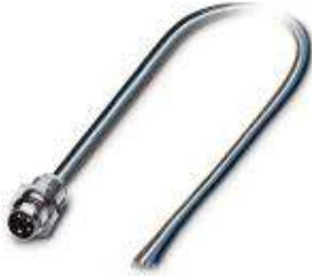
Sensor/actuator flush-type plug, 4-pos., M8, front/screw mounting, with M8 thread, with 0.5 m TPE litz wire, 4 x 0.25 mm 2
