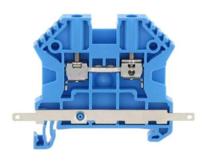
Feed-through terminal, Screw connection, Mounting type: Mounting rail TS 35/7.5, Rated cross-section: 2.5 mm², Width: 5 mm, Colour: Blue
