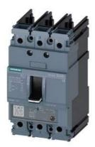
circuit breaker 3VA5 UL frame 125 breaking capacity class S 25kA @ 480V 3-pole, line protection TM230, FTAM, In=35A overload protection Ir=35A fixed short-circuit protection Ii=5...10 x In UL 489 SB (naval), 50° C without connection
