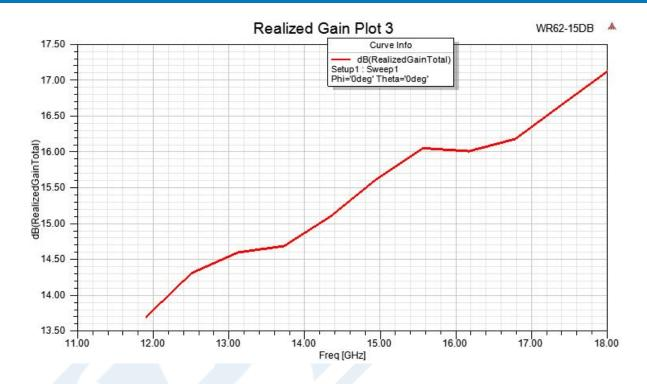
Click the following link (or enter part number in "SEARCH" on website) to obtain additional part information including price, inventory and certifications: WR-62 Standard Gain Horn with 15 dBi gain, End Launch SMA Female connector PEWAN062-15ELSF
