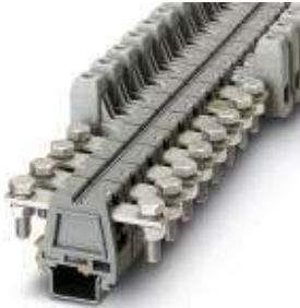
Universal terminal block with bolt connection, cross section: 6 - 25 mm 2 , AWG: 10 - 4, width: 26 mm, color: Gray
