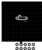
a. 60^\circ\text{C}/\text{W} when mounted on a 1 in 2 pad of 2 oz copper
