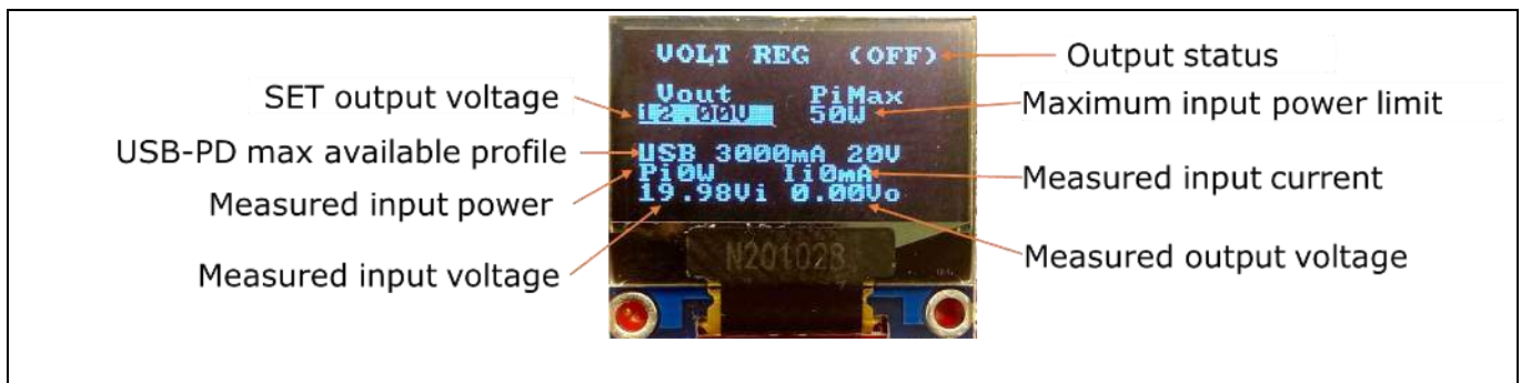
Figure 13 TLD5542-1VOLTAGE sketch, main screen
