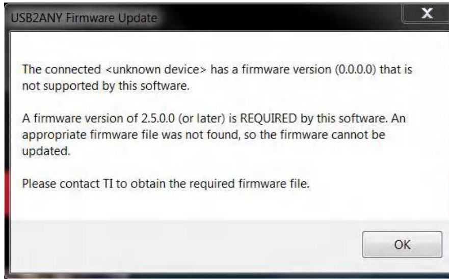
Figure 3-26. Error That States That USB2ANY Firmware Must be Updated
