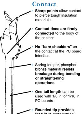
lead-in to mate with PC board holes
