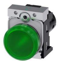
Indicator lights, compact, 22 mm, round, metal, green, lens, smooth, with holder, Operating voltage 24 V AC/DC, screw terminal
