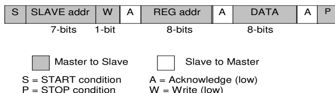
Figure 24: I 2 C Byte Write (SDA line)
