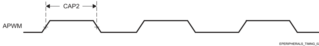
Figure 7-42. eCAP Switching Characteristics
