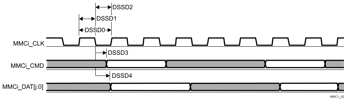
Figure 7-73. eMMC/SD/SDIO in - Default Speed - Transmitter Mode
