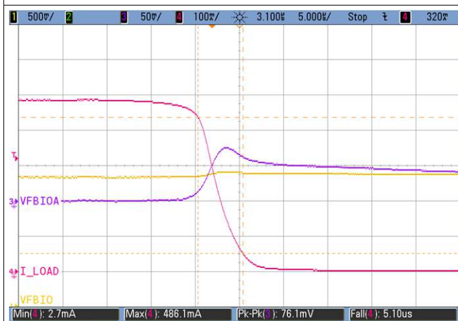
VCCIO = 3.8 V Vout = 1.8 V PWM Mode Figure 7-6. VDDIO Falling Load Transient Response
