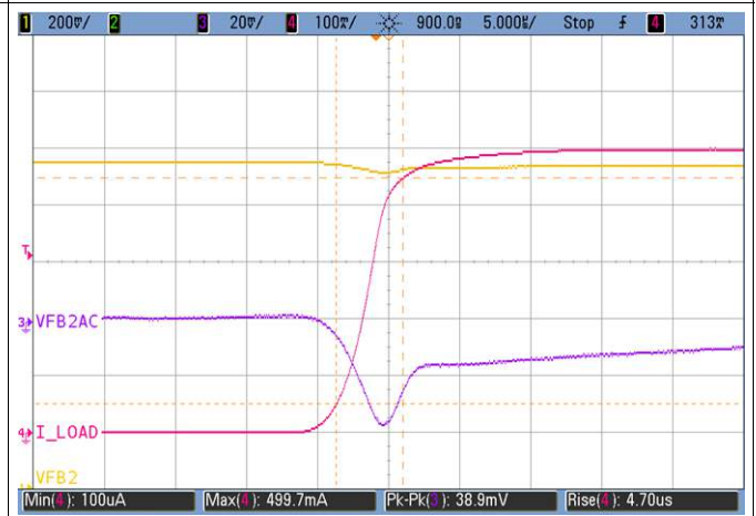
VCC2 = 3.8 V Vout = 1.2 V PWM Mode Figure 7-5. VDD2 Rising Load Transient Response
