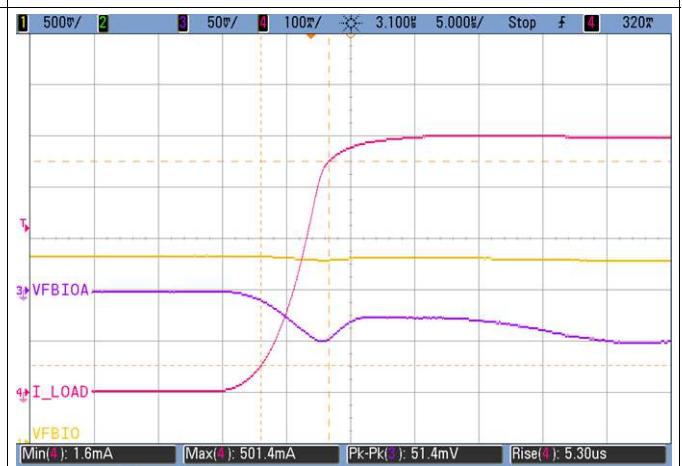
VCCIO = 3.8 V Vout = 1.8 V PWM Mode Figure 7-7. VDDIO Rising Load Transient Response
