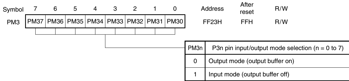
Figure 13-3. Format of Port Mode Register 3
