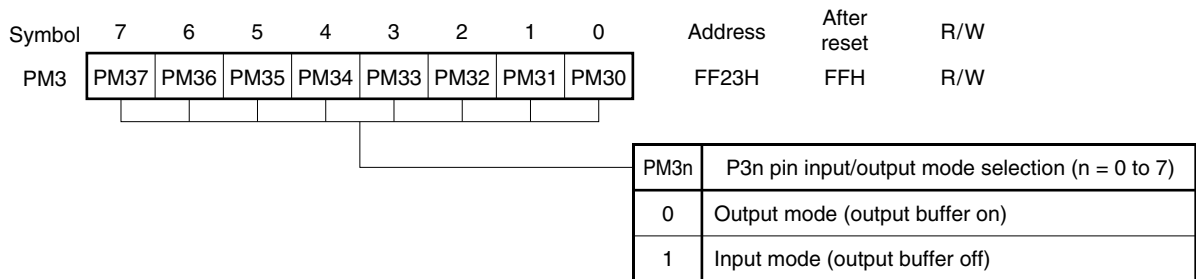
Figure 12-4. Format of Port Mode Register 3
