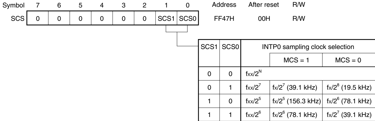
Figure 21-7. Format of Sampling Clock Select Register
