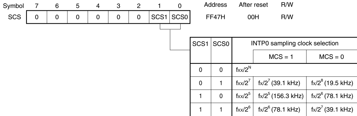
Figure 8-9. Format of Sampling Clock Select Register
