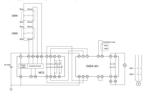
KM1, KM2: Magnetic contactor M: Motor
