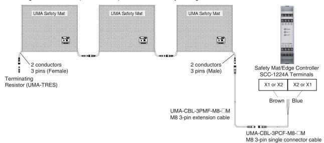
• Connecting three 2-cable Mats (UM□□A-□-□-2) to a MC3 Safety Mat Controller.
