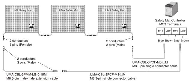
Note: 1. When an MC3 is used, the total cable length is up to 100 m and up to 12 Safety Mats can be connected (up to 10 m² in total). When an SCC-1224A is used, the total cable length is up to 25 m and up to 10 Safety Mats can be connected (up to 10 m² in total). For the 1-cable type of UMA Safety Mat (UM A----1), the total lone length of cable must be calculated by multiplying the total length of the cables used by two.
