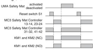
Note: Remove the three yellow jumpers from the MC3 to use Manual Reset Mode. Refer to Changing the Reset Mode on page 10 for the location of the jumpers.
