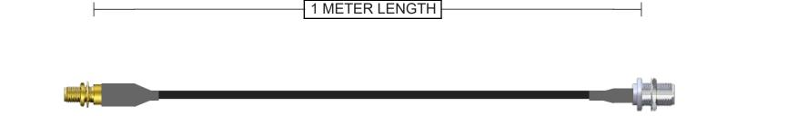
Connector A 132453 SMA Jack Straight Bulkhead - Rear Mount Brass Gold + Heatshrink 50 Ohm LMR-240 Continuity/Hi-Pot Connector B 172386 N-Type Jack Straight Bulkhead - Rear Mount Brass White Bronze + Heatshrink
