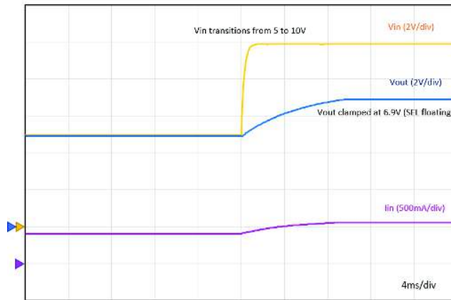
Figure 5. Output Voltage Protection
