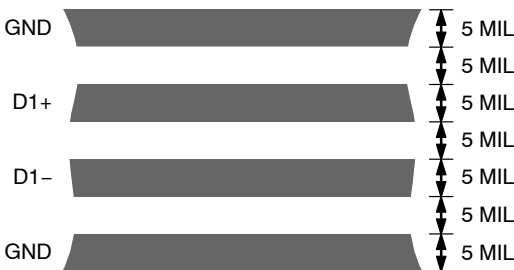
Figure 17. Arrangement of Signal Tracks
