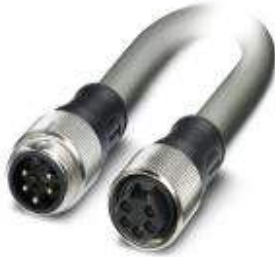
Bus system cable, DeviceNet, 5-position, PVC, Gray RAL 7001, Plug straight 7/8"-16UNF, on Socket straight 7/8"-16UNF, Cable length: 0.5 m
