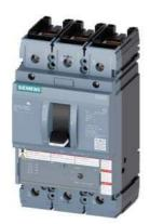
circuit breaker 3VA5 UL frame 250 3-pole, starter protection TM120M, AM, In=150A without overload protection short-circuit protection Ii=6...12 x In cable connection on both sides
