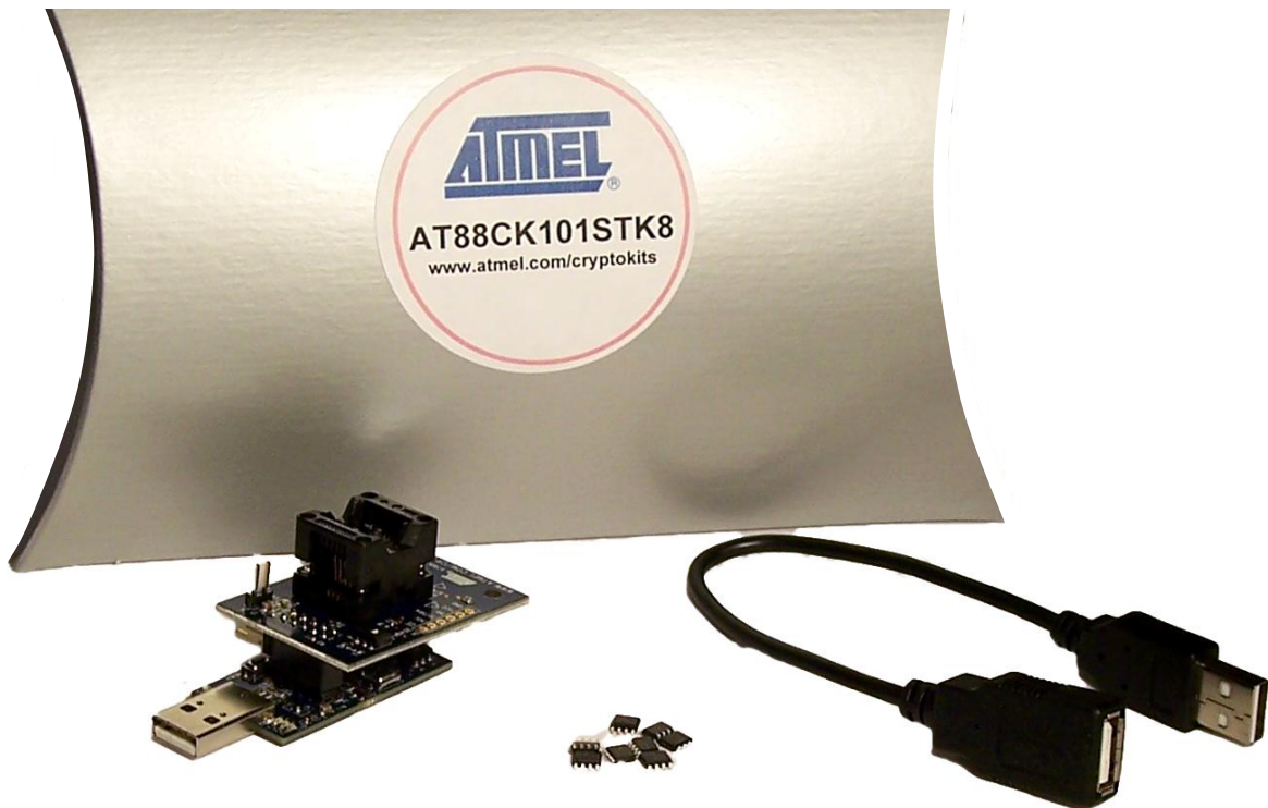
Figure 1. Atmel AT88CK101STK8 starter kit
