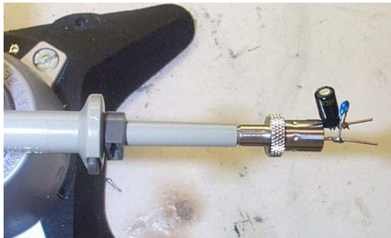
Figure 58 – Oscilloscope Probe with Probe Master 4987BA BNC Adapter (Modified with Wires for Probe Ground for Ripple measurement and Two Parallel Decoupling Capacitors Added).
