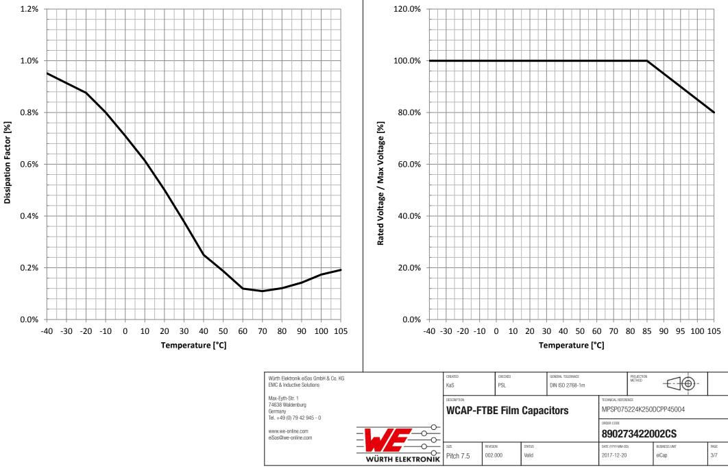
**Rated Voltage vs. Temperature:**
