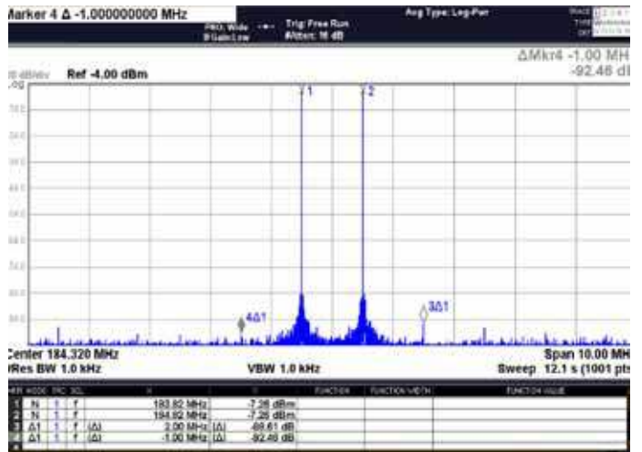
Fig 10. IMD3 (dBc) for two tones (spacing 10 MHz) centered at 184.32 MHz
