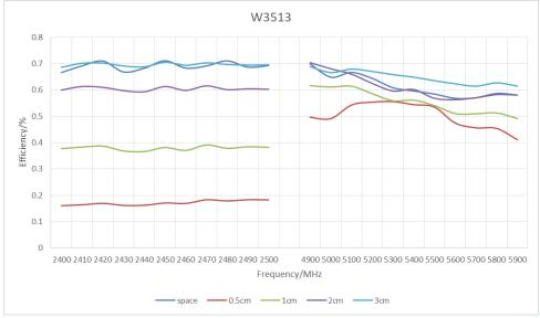
When the distance is 0.5-2cm, the metal mainly affect the performance of low frequency band(2.4G-2.5G). When the distance is above 2cm,the metal will have a little influence in two band.
