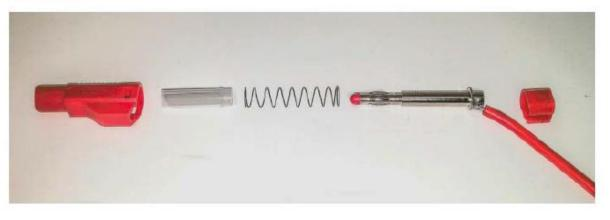
Note: Use very short wire strip length and solder just above the spring retainer.
