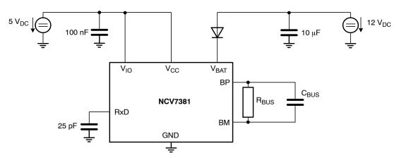
Figure 17. Test Setup for Dynamic Characteristics
