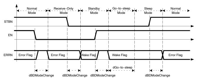
Figure 4. Timing Diagram of Operating Modes Control by the STBN and EN Pins
