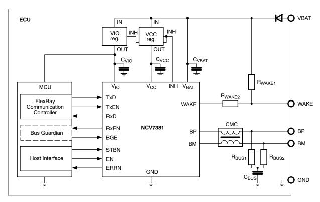
Figure 2. Application Diagram
