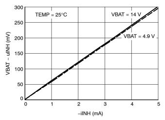
Figure 16. INH Not\_Sleep Output Characteristic
