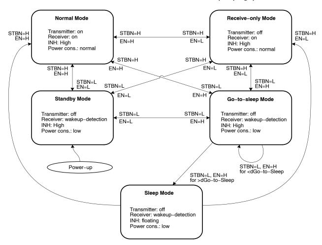
Figure 3. Operating Modes and their Control by the STBN and EN Pins
