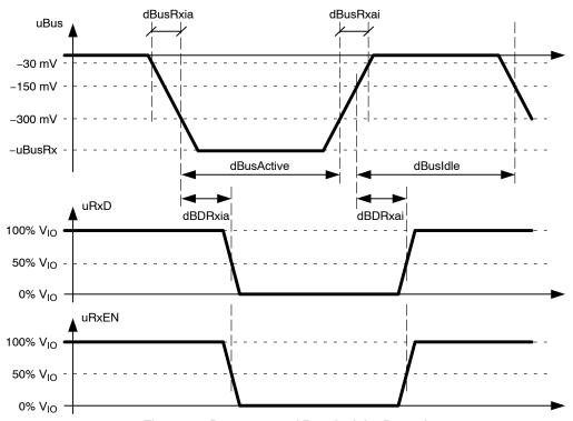
Figure 13. Parameters of Bus Activity Detection
