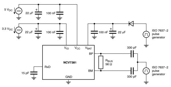
Figure 18. Test Setup for Measuring the Transient Immunity
