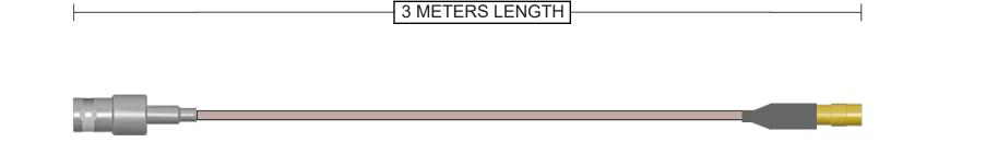
Connector A 112160 BNC Jack Straight Brass Nickel 50 Ohm RG-316 Continuity/Hi-Pot Connector B 262118 MMCX Jack Straight Brass Gold + Heatshrink
