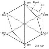
Sample: G6BK-1114P-US Number of Relays: 12 pcs Test Conditions: The value at which malfunction occurred was measured after applying shock to the Shock direction test piece 3 times each
