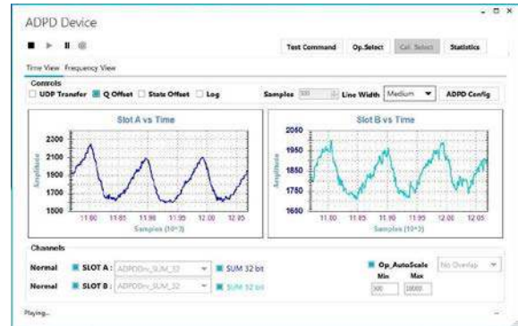
Figure 23. Reflectance PPG Taken Using the Example SpO2 Setup File (see Table 12) Programmed Through Analog Devices Wavetool Software
