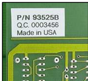
Circuit board labeling
