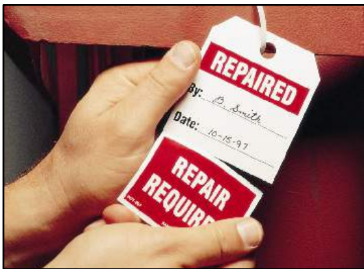
Sign tag and tear at perforation once the status has changed
