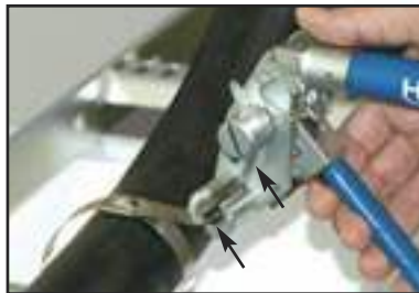
Position the CT-7 in loading position (ratchet handle forward) then place the band through Tool Nose and Winding Mandrel. Make sure there is plenty of band through the Mandrel.
