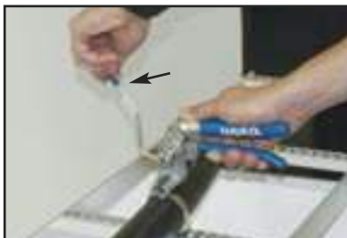
Push forward the Cutter Handle to trim the band.
