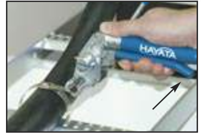
Grip Ratchet Handle and pull back toward Handle to tighten band.
