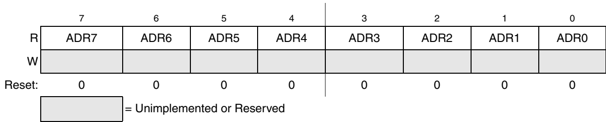
Figure 8-7. Data Result Low Register (ADCRL)
