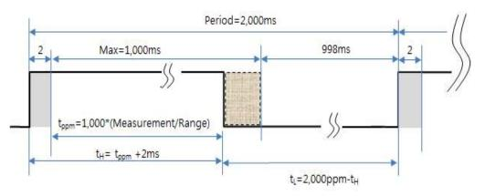
EX)  $t_H$ (High Pulse Width) calculation for 400ppm in 2,000 ppm Range. \*Measurement<sub>(ppm)</sub> = 400 ppm = ( $t_H$ -2ms)/2,000msec x Range<sub>(ppm)</sub> , \* $t_H$ = 1,000 msec \* (400 ppm / 2,000ppm) + 2msec = 202msec (cf:  $T_L$ = Period -  $t_H$  = 2,000ppm - 202 msec = 1,798 msec.)
