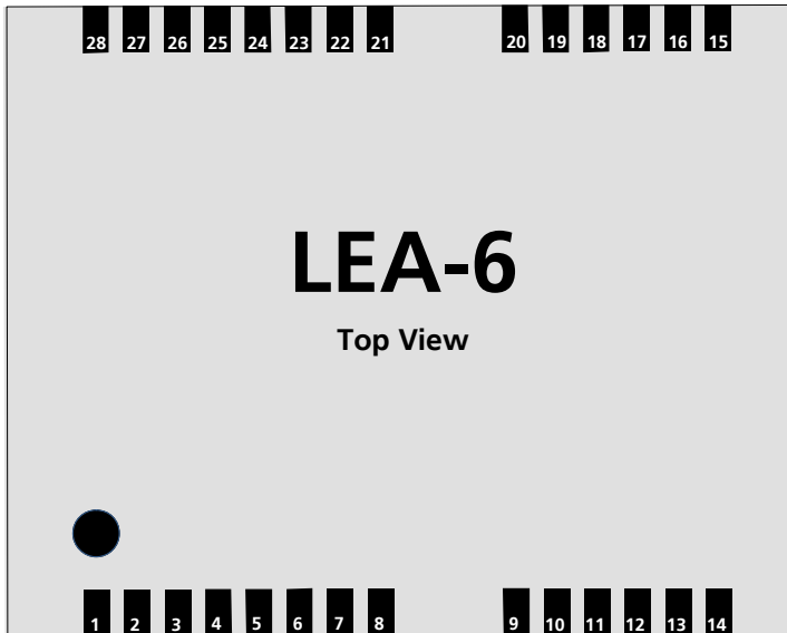
Figure 2 LEA-6 Pin Assignment
