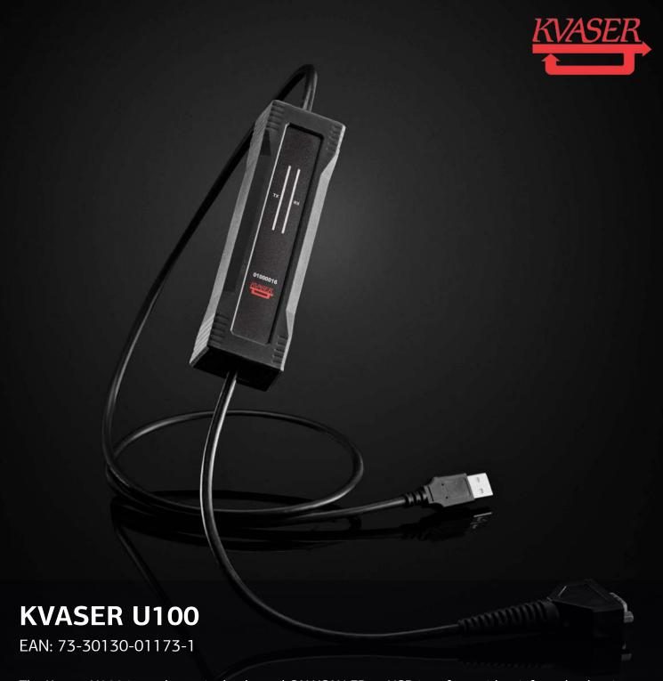
The Kvaser U100 is a robust, single-channel CAN/CAN FD to USB interface with reinforced galvanic isolation that squarely addresses the needs of the evolving automotive development market. Fully compatible with J1939, CANopen, NMEA 2000® and DeviceNet, this is the first in a new range of interfaces that is also suited to rugged applications in marine, industrial, heavy duty vehicle and heavy industries.
