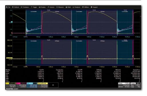
errors and the measurement parameters provide details of single cycle or average device power losses. Beyond the advanced power loss measurement capabilities, the Power Analyzer modulation analysis capabilities provide insight to understand control loop response to critical events such as a power supply's soft start performance or step response to line and load changes.
