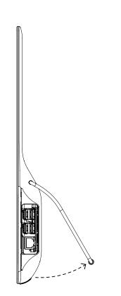
Plug in the Power Supply and hold the Power Button beside it for 2-3 seconds to turn on your  $\mbox{{\bf pi-top}}\mbox{\sf CEED}.$
