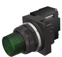
30mm BlackMax, Epoxy Coated Corrosion Resistant Complete Metal Unit Illuminated Indicator Light Transformer type, 600V AC Incandescent Lamp, BA9s Glass Lens, Green UL Listed, CSA Certified NEMA 1,3,3R,4,4X,12,13 & Automotive Standards
