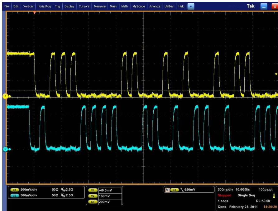
Figure 5. EMI4193 MIPI D-PHY LP Mode Measured Results
