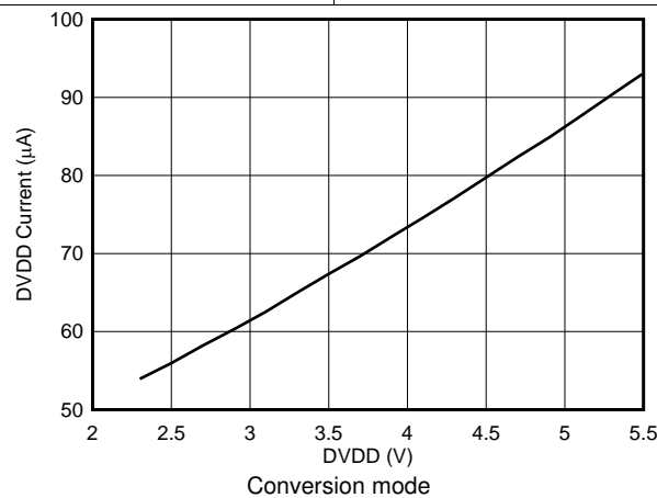
Figure 26. Digital Supply Current vs DVDD
