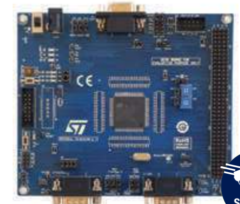
Discovery Kit for the L Line with SPC56EL70L5. order code: SPC56EL70L5DISP
