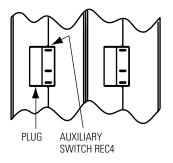
Alarm & Auxiliary Switch Combination
