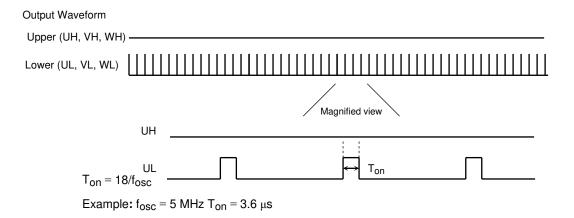
(2) If the VSP input voltage is 2.1 V < VSP and the Hall signal is 5 Hz or less, the upper phase (UH, VH, WH) will perform 120° energization at a PWM that complies with the VSP; and the lower phase (UL, VL, WL) will operate at 120° energization, performing refresh operation based on the OFF timing. (The same drive is executed during reverse rotation as well.)</p>
