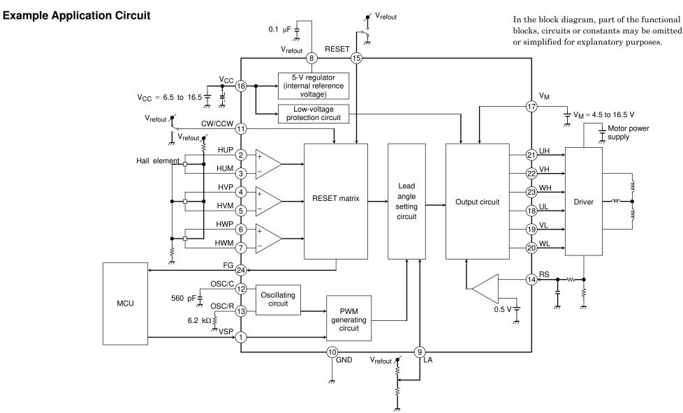
Note: Utmost care is necessary in the design of the output, V<sub>CC</sub>, V<sub>M</sub>, and GND lines, since the IC may be destroyed by short-circuiting between outputs, short to VCC, short to VM or short to ground.
