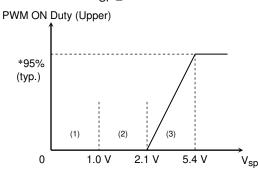
\*: The maximum ON duty is  $T_{on} = 95\%$  (typ.) when  $V_{SP} = 5.4 V$  (typ.). Example: If  $f_{OSC} = 5 \text{ MHz}$ , then ON time = 48 µs (typ.) ( $f_C = 19.8 \text{ kHz}$ ) If  $f_{OSC} = 4 \text{ MHz}$ , then ON time = 60 µs (typ.) ( $f_C = 15.9 \text{ kHz}$ )
