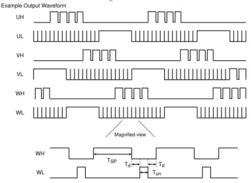
$T_{SP}$ : Variable depending on the  $V_{SP}$  (the figure above being applicable when  $V_{SP} = 5.4$  V (typ.));  $T_{on} = 18/f_{osc}$ ;  $Td = 18/f_{osc}$
