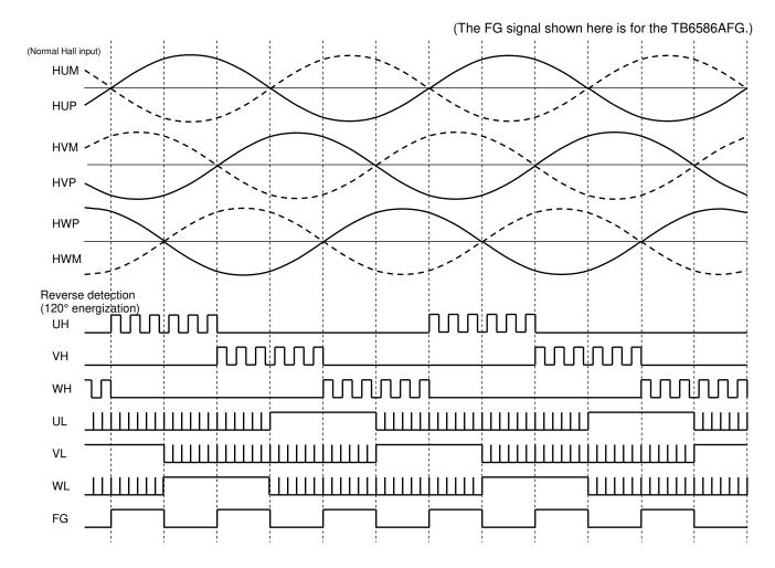
\*: When CW/CCW = High and a normal Hall signal is input, it runs at 120° energization for a lead angle of 0° (reverse rotation).
