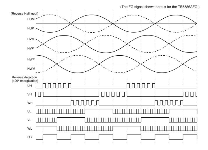
\*: When CW/CCW = Low and a reverse Hall signal is input, the motor runs at 120° energization for a lead angle of 0° (reverse rotation)
