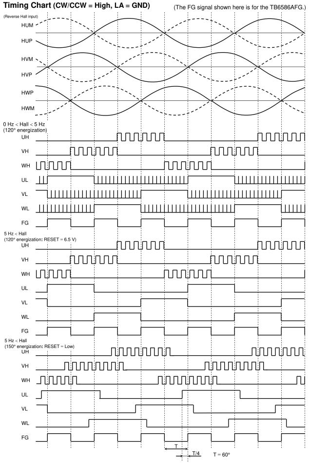
\*: When the Hall signal is 5 Hz or higher, the lead angle function operates in accordance with the LA pin signal.
